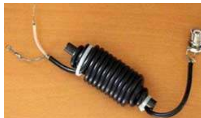
A 1:1 Guanella (current) balun, also known as a "choke", made by winding 3 layers of RG58 coax on a ferrite rod.
