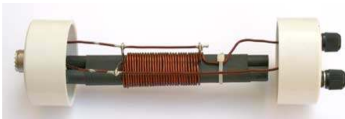
A 4:1 Ruthroff (voltage) balun wound on ferrite rods, using laquered wire. For more bandwidth the spacing between the windings should be increased. This balun will take at least 100W.
