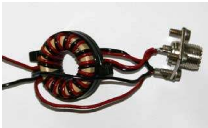
A 4:1 Guanella (current) balun on a single toroid, made from insulated wire and cable ties.
