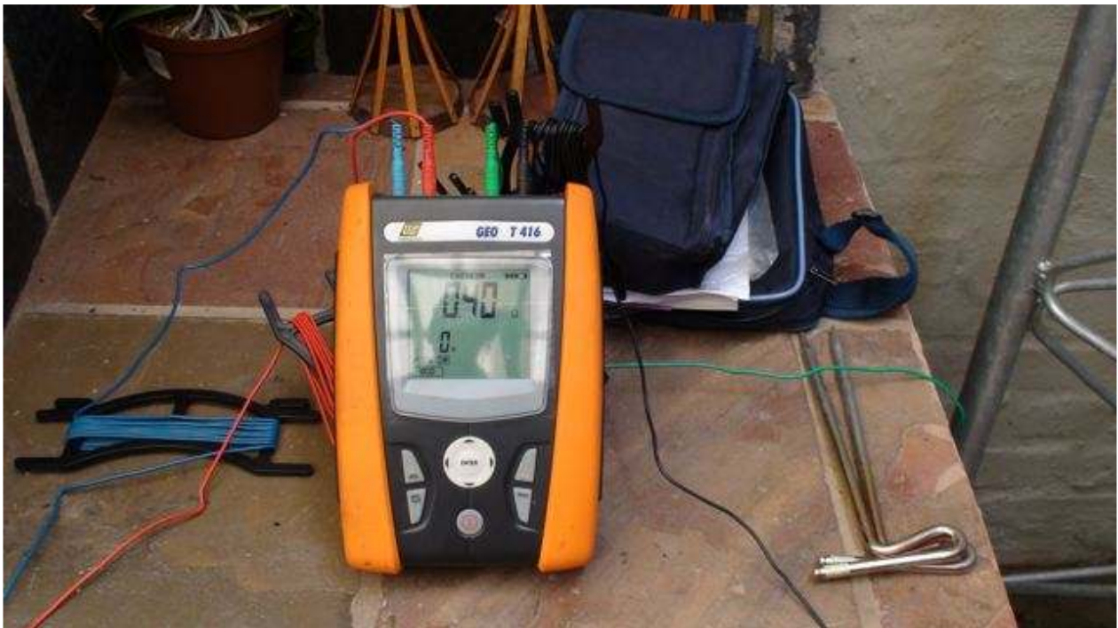
One of the lowest measurements as opposed to 0,43 ohms measured in a second test. The equipment is a sophisticated GEO T416 3-point measurement system.
