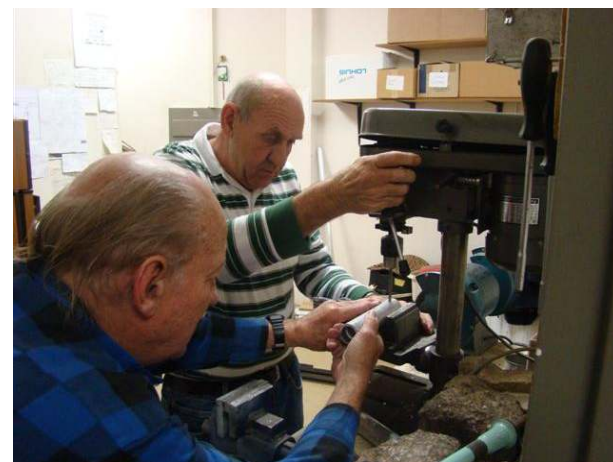
Alf and Whitey drilling tubing for centre support
