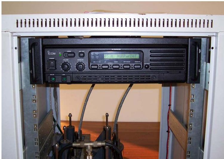
ICOM FR-3000 (remote controllable) just above the duplexer.
