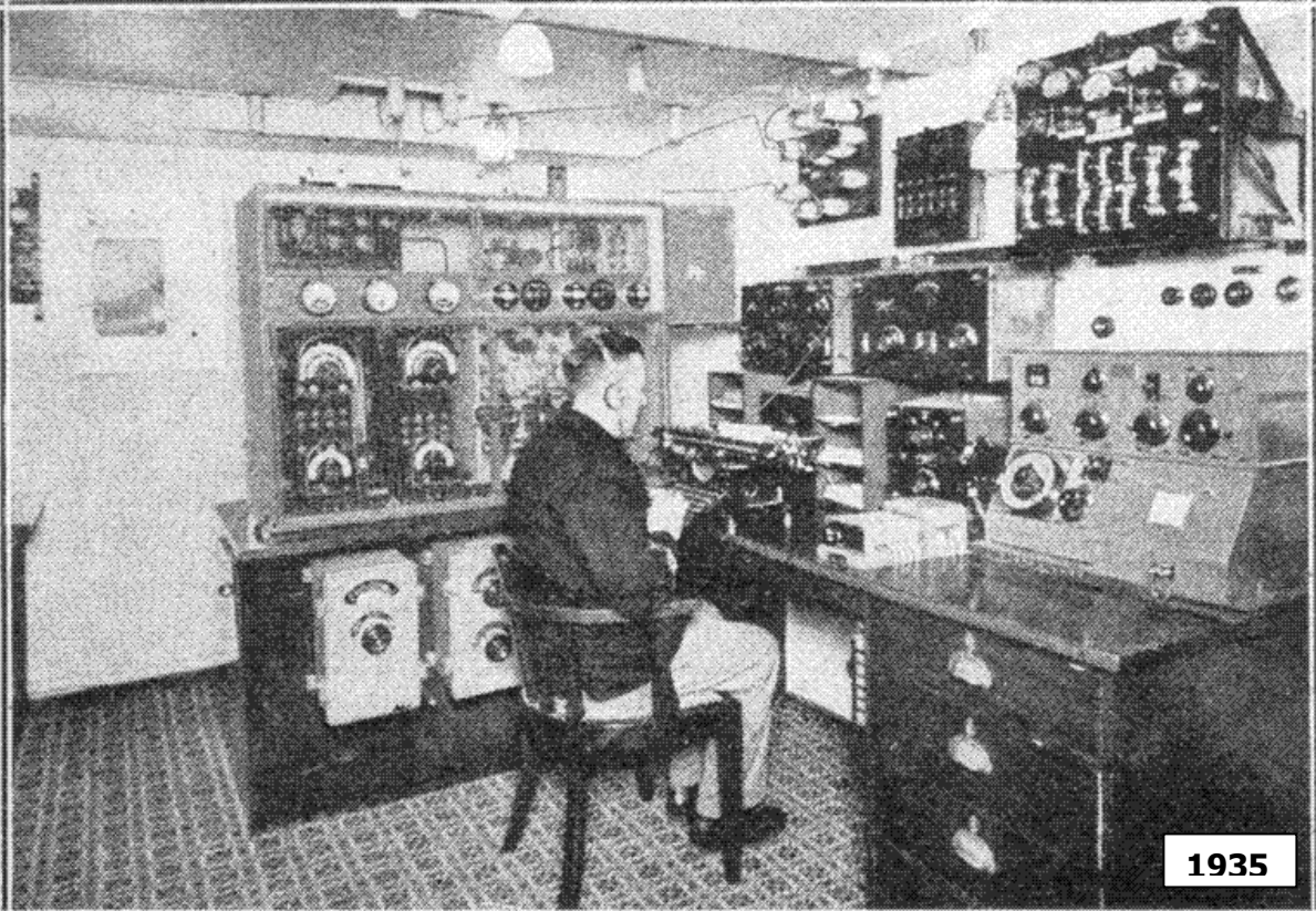
The elaborate Marconi Wireless transmitting and receiving apparatus installed on the "Empress of Britain."
